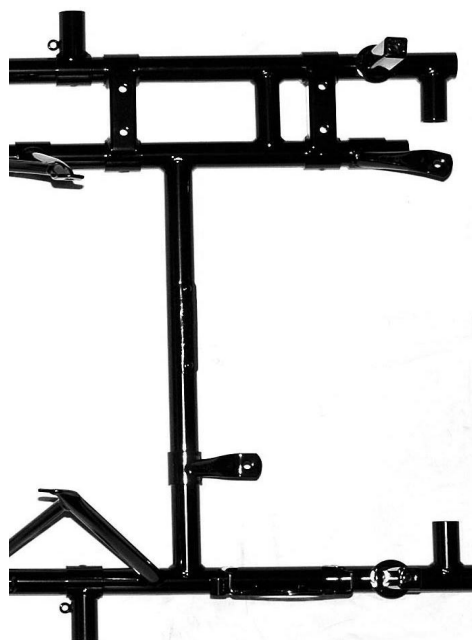
Foto from above of the frame with the section of the two supports for the RTPS (Rear Tire Protection System)
