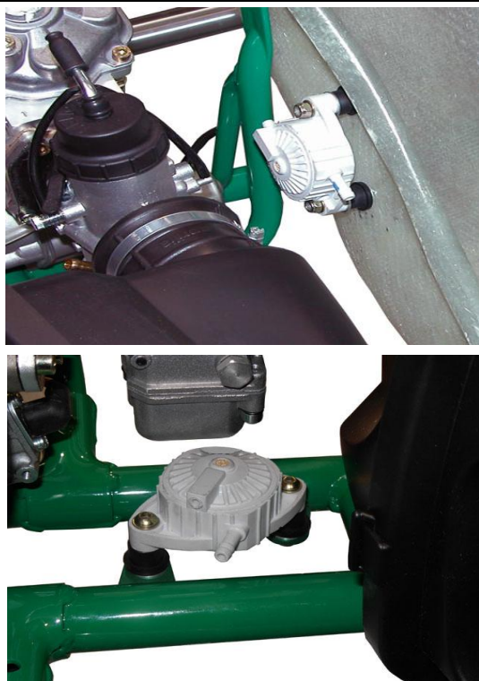
Photo of the frame with the section of the support for the fuel pump (fuel pump mounted)
