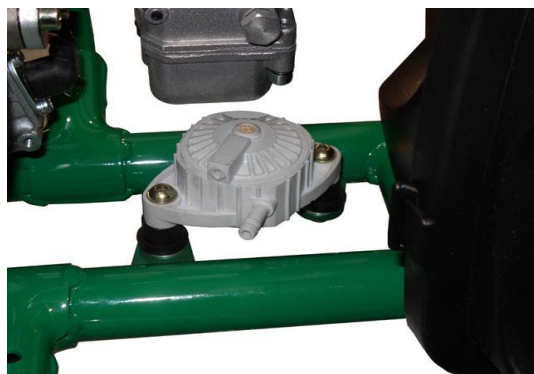
Photo of the frame with the section of the support for the fuel pump (fuel pump mounted)
