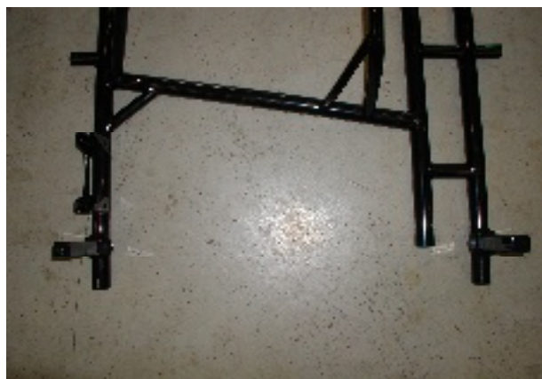
Photo from above of the frame with the section of the two supports for the RTPS (Rear Tire Protection System)
