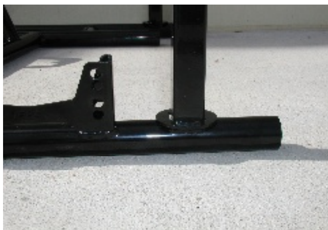
Photo of the frame from the side with the section of the support for the RTPS (Rear Tire Protection System)
