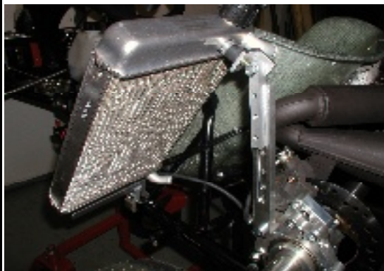
Foto of the frame from the side with the section of the supports for the radiator (radiator mounted)
