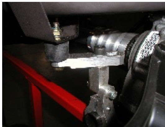
Photo from above of the frame with the section of the two supports for the exhaust system
