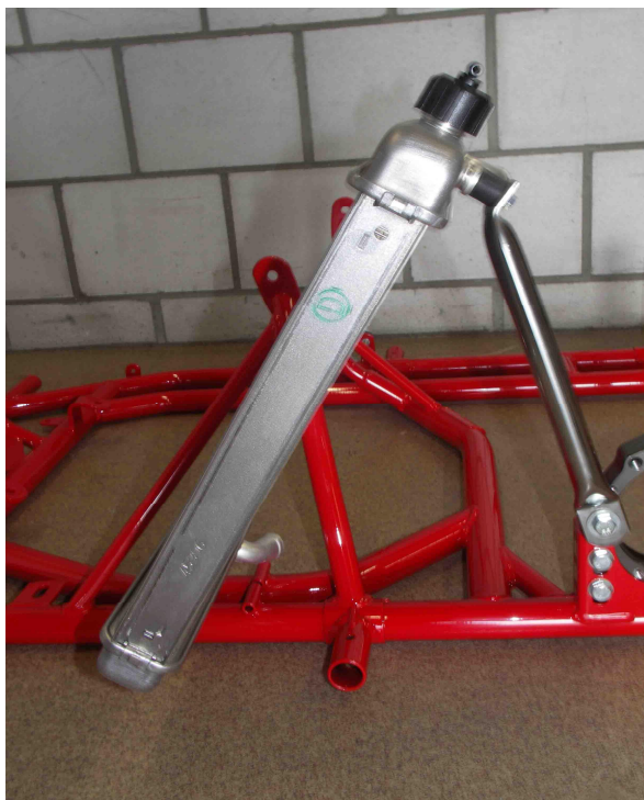
Photo of the frame from the side with the section of the supports for the radiator (radiator mounted)
