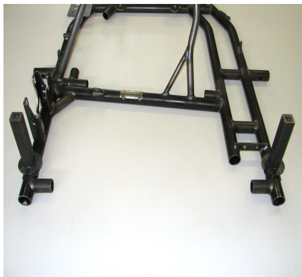
Photo from above of the frame with the section of the two supports for the RTPS (Rear Tire Protection System)
