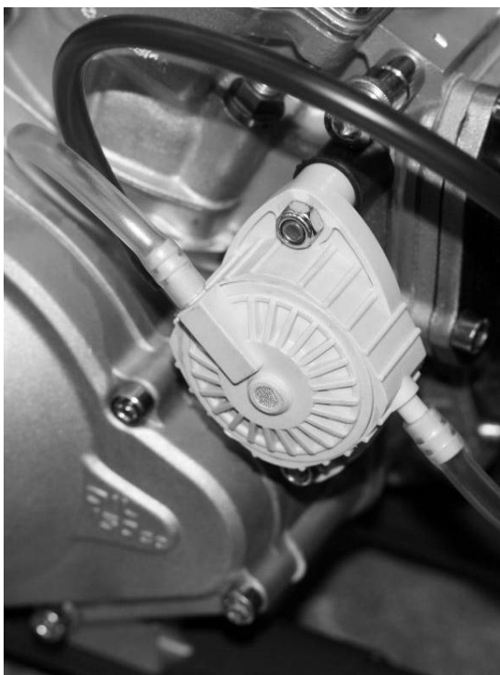
Foto of the frame with the section of the support for the fuel pump (fuel pump mounted)
