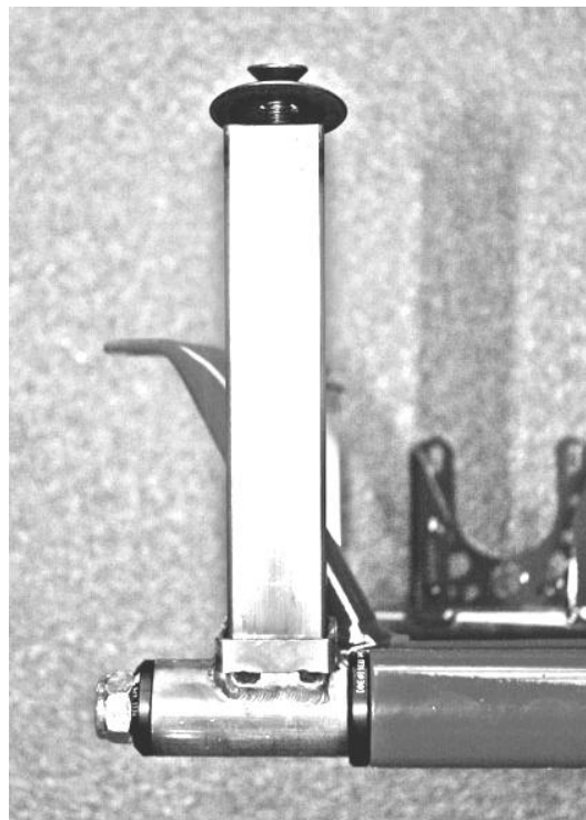
Foto of the frame from the side with the section of the support for the RTPS (Rear Tire Protection System)
