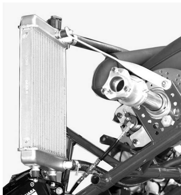
Foto of the frame from the side with the section of the supports for the radiator (radiator mounted)
