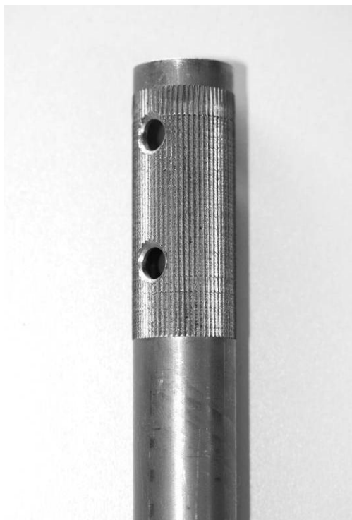
Foto from the steering column with the section with the knurling for the steering wheel hub (knurling according to DIN 82 - RAA1).
