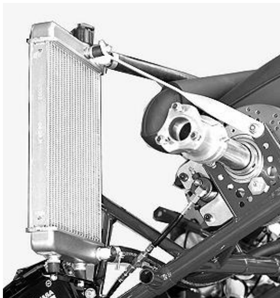
Photo of the frame from the side with the section of the supports for the radiator (radiator mounted)
