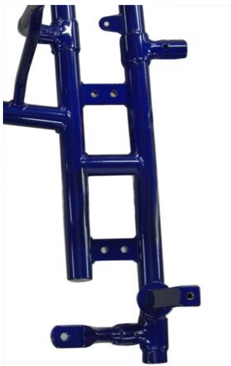
Photo from above of the frame with the section of the engine mount
