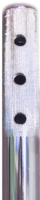
Photo from the steering column with the section with the knurling for the steering wheel hub (knurling according to DIN 82 - RAA1).
