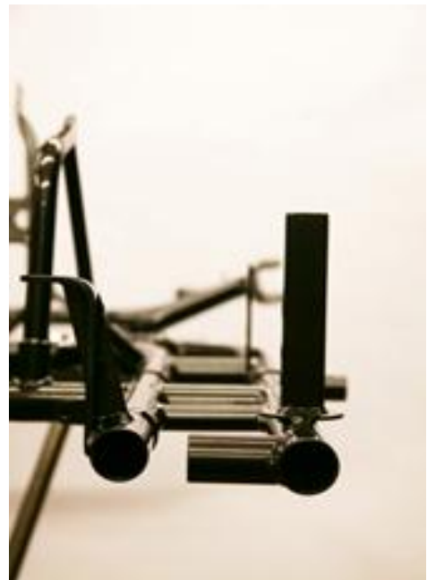
Photo of the frame from the back with the section of the support for the RTPS (Rear Tire Protection System)
