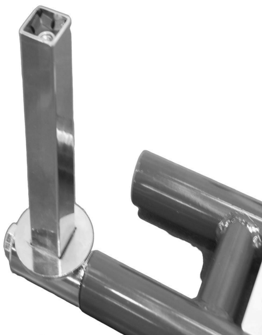
Photo of the frame from the back with the section of the support for the RTPS (Rear Tire Protection System)
