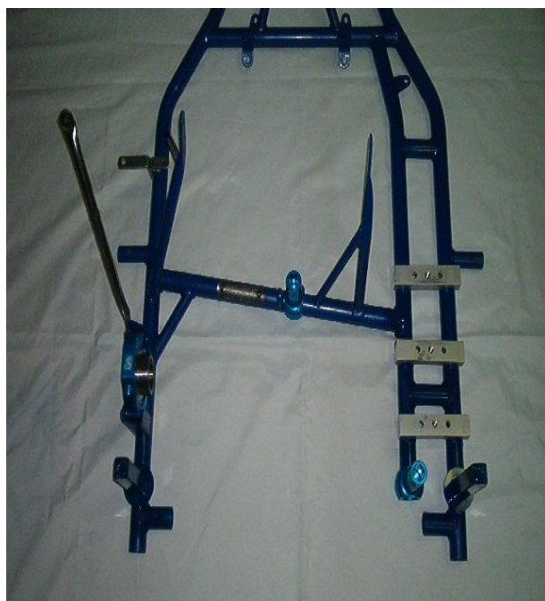
Photo from above of the frame with the section of the two supports for the exhaust system
