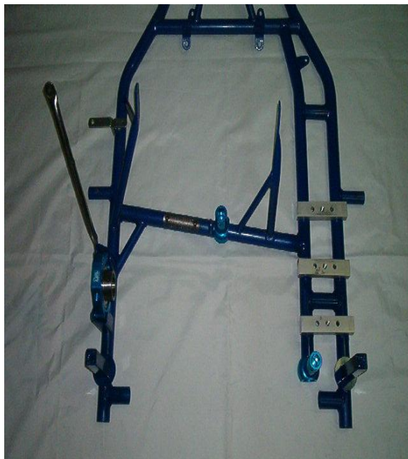
Photo from above of the frame with the section of the two supports for the RTPS (Rear Tire Protection System)
