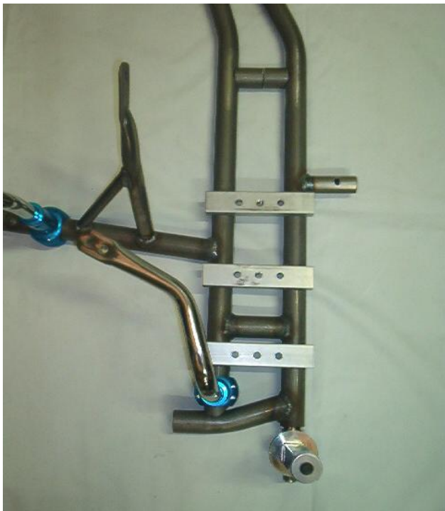
Photo of the frame from the side with the section of the support for the RTPS (Rear Tire Protection System)
