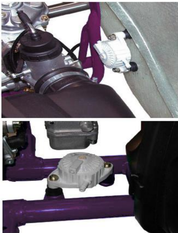
Photo of the frame with the section of the support for the fuel pump (fuel pump mounted)
