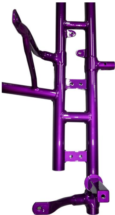
Photo from above of the frame with the section of the engine mount
