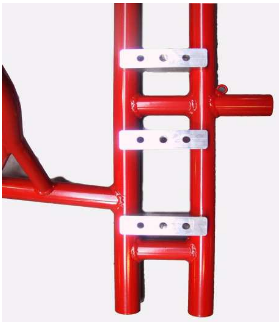
Above: photo of the frame with the section of the engine mount
