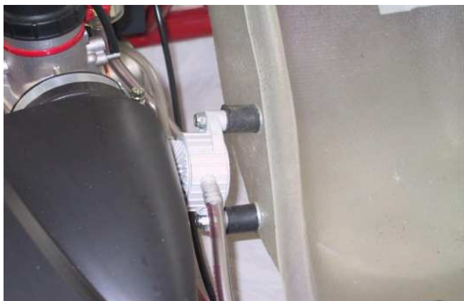
Above: Photo of the frame with the section of the support for the fuel pump (fuel pump mounted)
