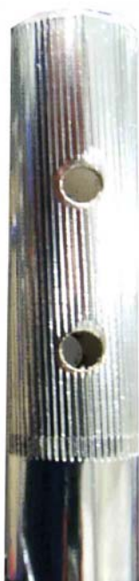
Foto from the steering column with the section with the knurling for the steering wheel hub (knurling according to DIN 82 - RAA1).
