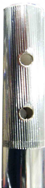
Foto from the steering column with the section with the knurling for the steering wheel hub (knurling according to DIN 82 - RAA1).
