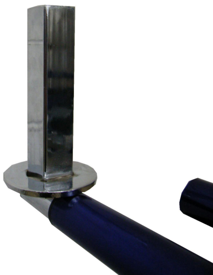
Photo of the frame from the side with the section of the support for the RTPS (Rear Tire Protection System)
