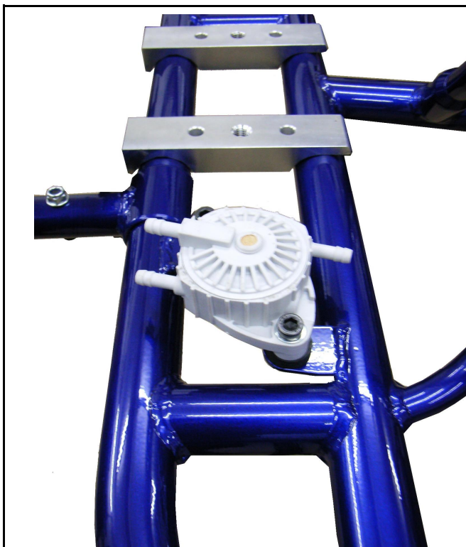
Photo of the frame with the section of the support for the fuel pump (fuel pump mounted)
