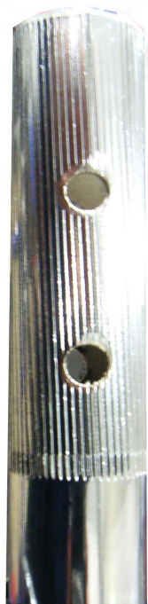
Photo from the steering column with the section with the knurling for the steering wheel hub (knurling according to DIN 82 - RAA1).
