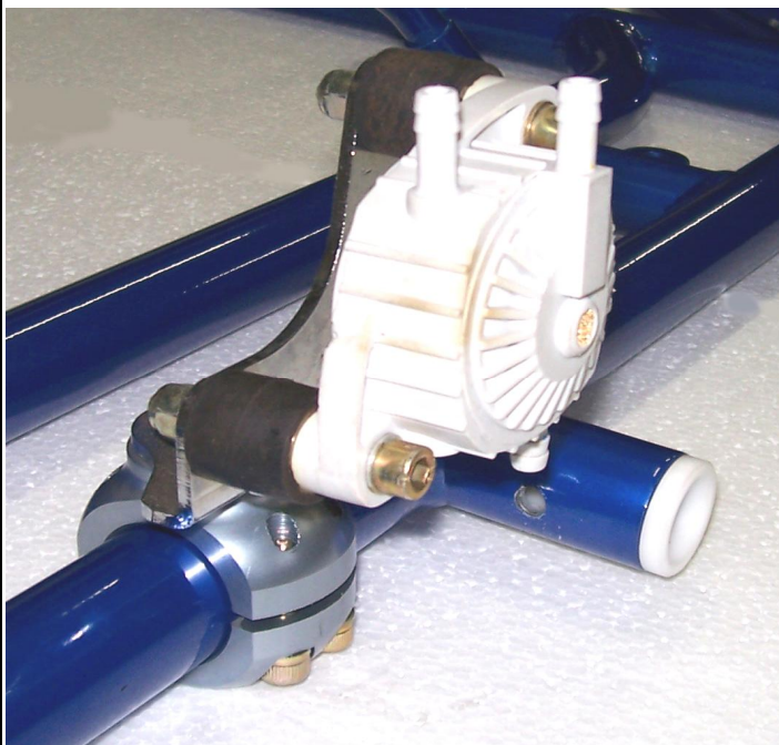
Photo of the frame with the section of the support for the fuel pump (fuel pump mounted)
